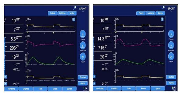
Yellow curve: Pressure (cmH<sub>2</sub>O) on X-axis and Time (seconds) on Y-axis Pink curve: Flow (L/sec) on X-axis and Time (seconds) on Y-axis Green curve: Tidal volume (ml) on X-axis and Time (seconds) on Y-axis
