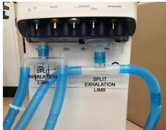
Figure 2: Final assembly of the coupler and Tee valve attached to the ventilator
