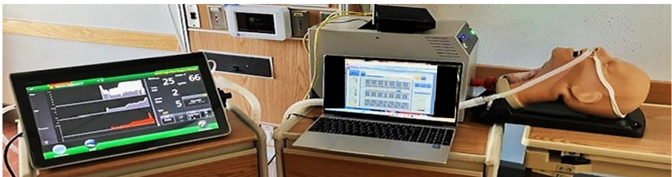
Figure 1 Setup of the experiment. On the left is the adaptive high-flow machine, while the right displays the ASL 5000 and mannequin.
