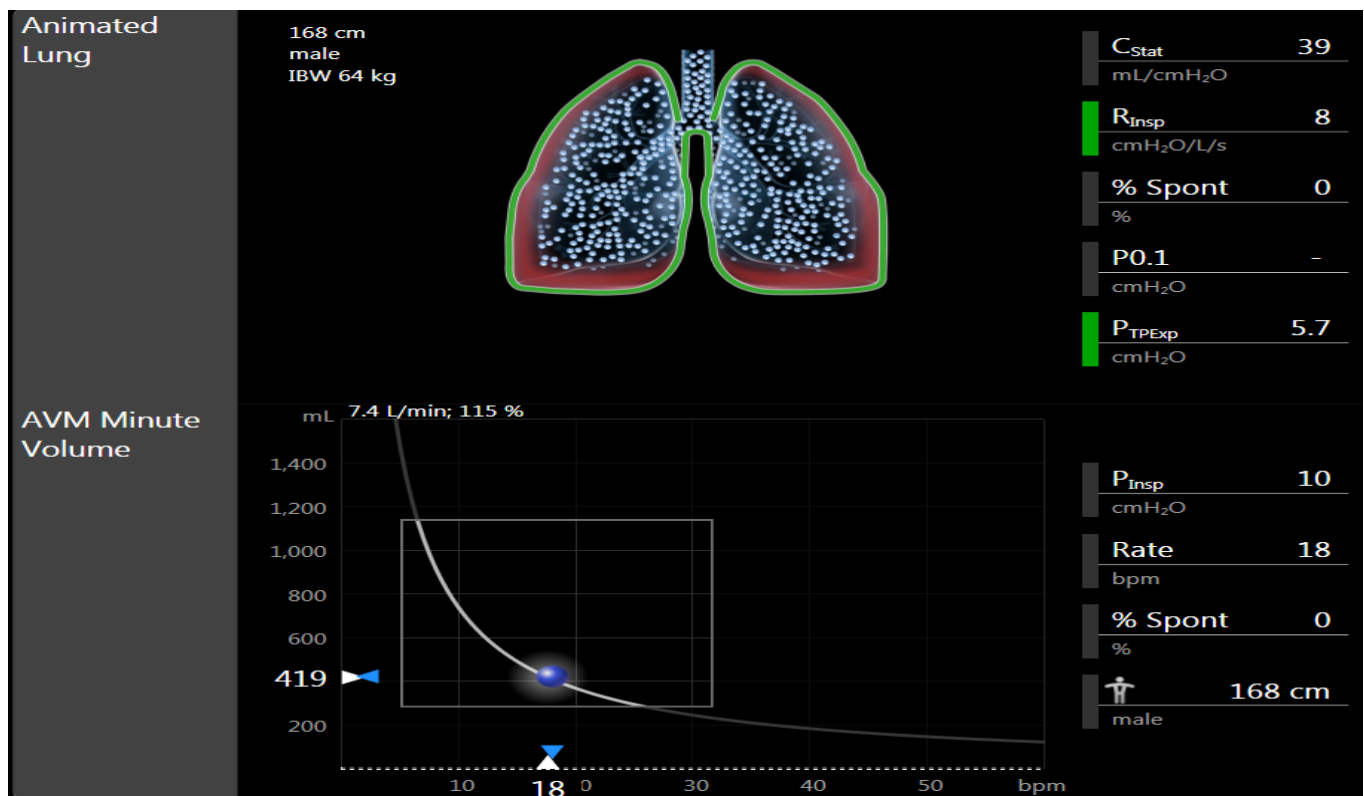
Figure 1: Top: animated lung showing height, gender and IBW, along with the corresponding compliance (Cstat), Inspiratory resistance (Rinsp), % Spontaneous effort, airway occlusion in 100 msec (P0.1), Expiratory trans-pulmonary pressure (PTPExp). Bottom is the AVM minute volume showing the % and target MV. Graph depicts the target respiratory rate (x-axis) vs tidal volume (y-axis) curve, blue circle and arrows indicate the optimal combination chosen by the ventilator.
