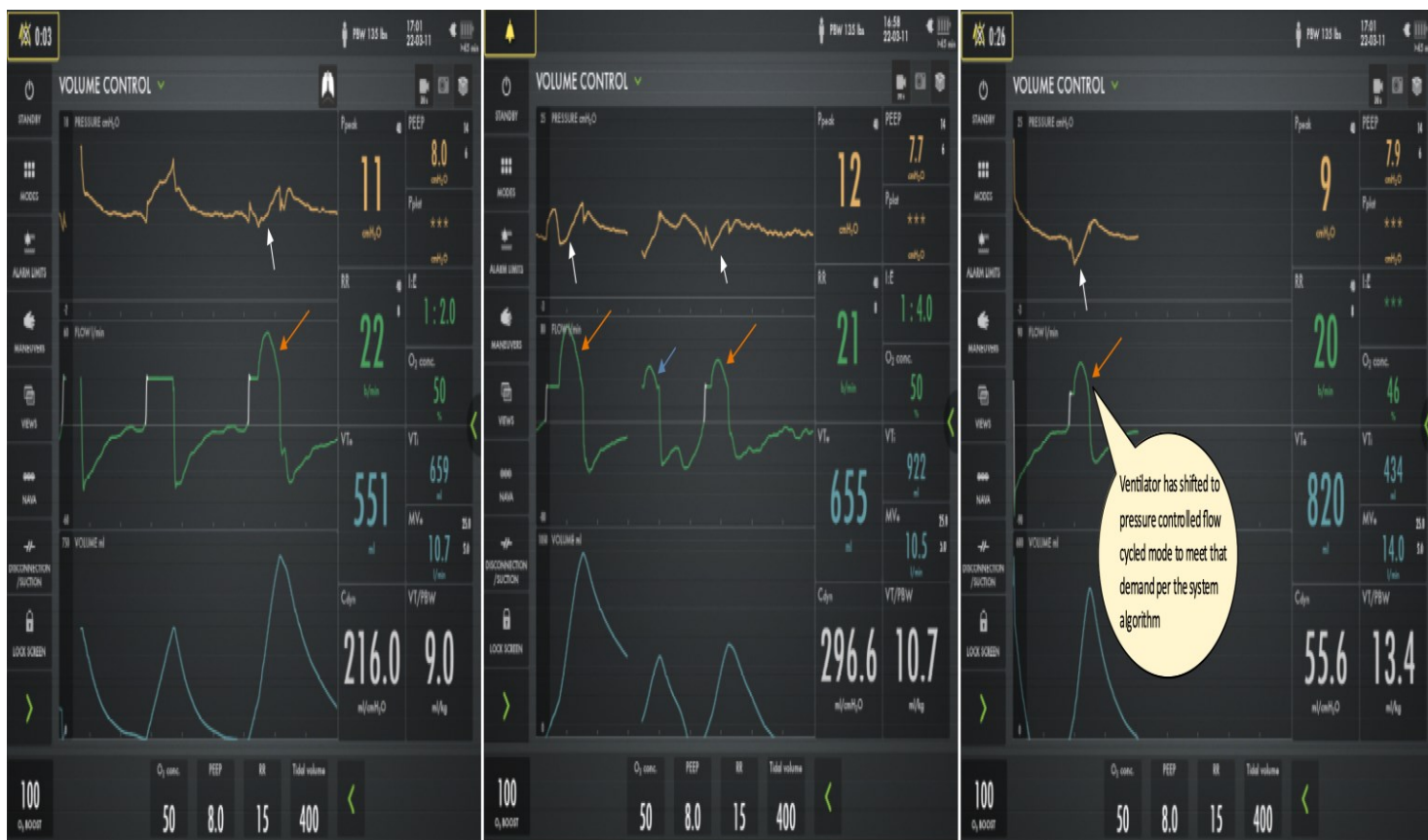
Figure 2: Volume control with adaptive flow tuned on, in an actively breathing patient. The white arrows show drop in pressure in response to patient efforts, resulting in individual mandatory breaths suppressed in dual targeting by switching volume cycling to flow cycling (orange arrows). The inspiration is prematurely interrupted once the set target volume is reached (blue arrow). Note increase in tidal volume shown as volume waveform peak value. Also note the variable inspiratory times as in Pressure Support
